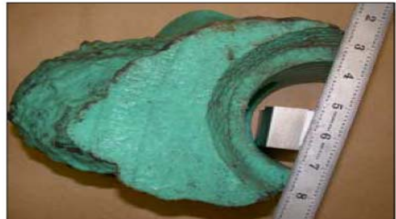
Rubberized Impression of Cavity
